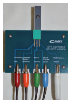
Figure 1.2. Left: Screen-printed electrode inserted into SPE cell stand. Right: Complete set-up.
