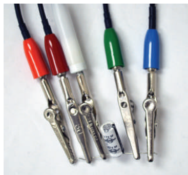
Single capacitor attached to potentiostat.
