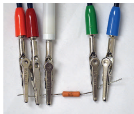
Single resistor attached to potentiostat.
