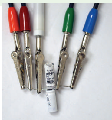
Capacitors in parallel attached to potentiostat.
