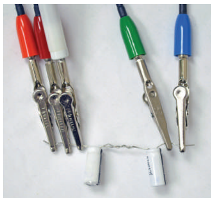
Capacitors in series attached to potentiostat.
