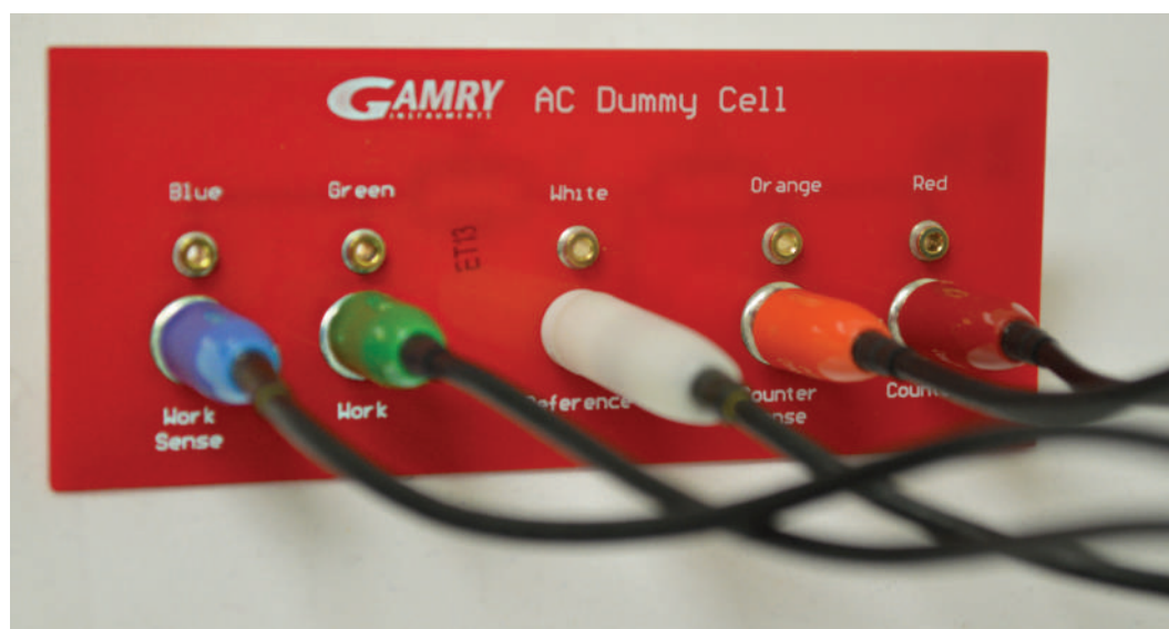
Figure 10.6. Connections from the Universal Dummy Cell (EIS Dummy Cell side) to the potentiostat.
