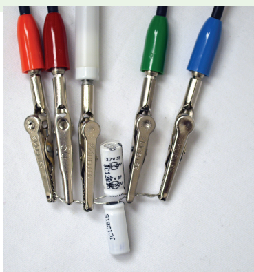
Capacitors in parallel attached to potentiostat.
