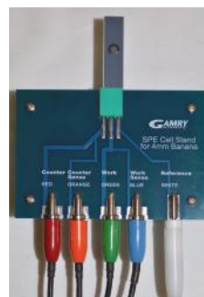
Figure 1.2. Left: Screen-printed electrode inserted into SPE cell stand. Right: Complete set-up.
