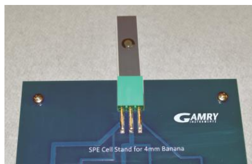
Figure 1.2. Left: Screen-printed electrode inserted into SPE cell stand. Right: Complete set-up.
