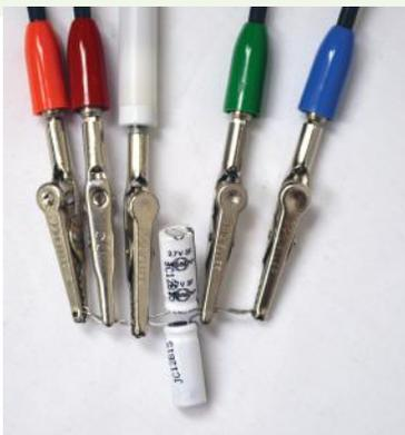
**Capacitors in parallel attached to potentiostat.**
